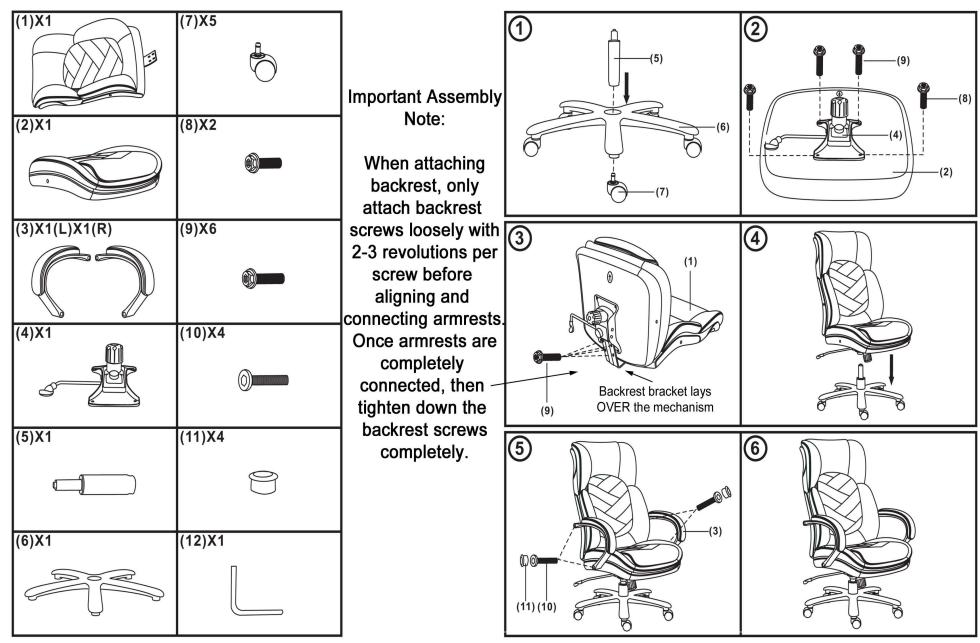
Screws are located in the holes. Use Allen Wrench to back them out for assembly.
