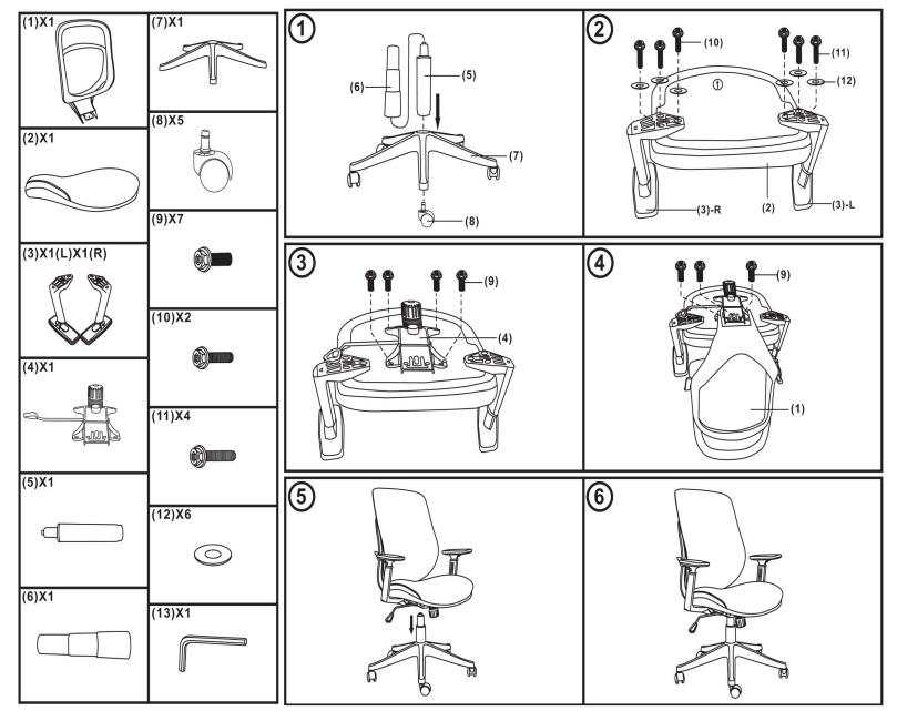
Screws and washers are located in the holes. Use Allen Wrench to back them out for assembly.
