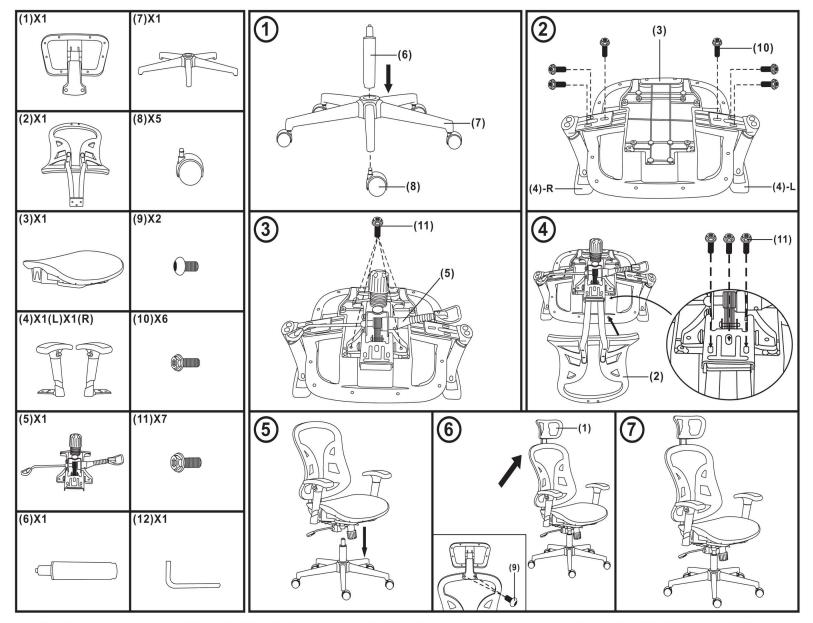
Mechanism screws located in holes on seat. Backrest screws are packaged with the gas lift.
