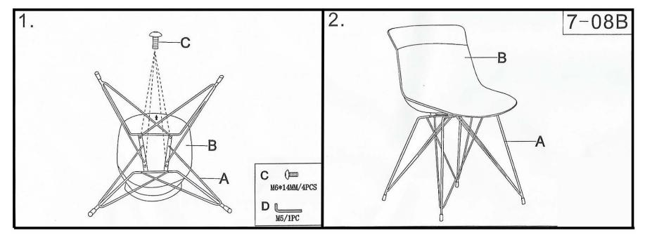
Step 1: Using Allen Wrench provided, attach A metal chair frame to B chair seat using four C screws.
