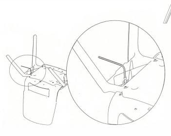
2.) If purchased with optional fabric padded seat, use a Phillips screwdriver to remove 10 Phillips screws from the underside of the seat. Remove the resin seat and replace with your padded seat. Reattach using the same screws.
