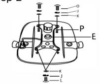
Attach (E) Mechanism to the (F) seat using the K, J, L, O and P hardware
