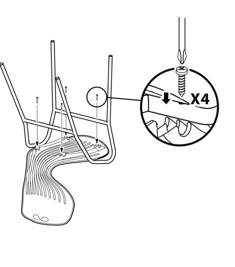
1.) Rest the shell upside down on a table for support during assembly. Insert screws as shown.
