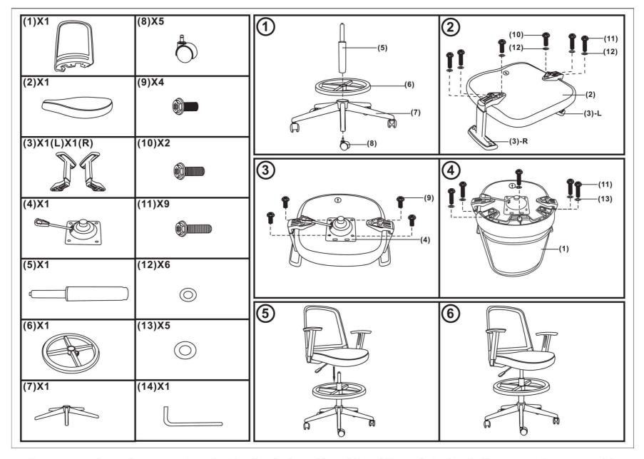
Screws and washers are located in the holes. Use Allen Wrench to back them out for assembly.
