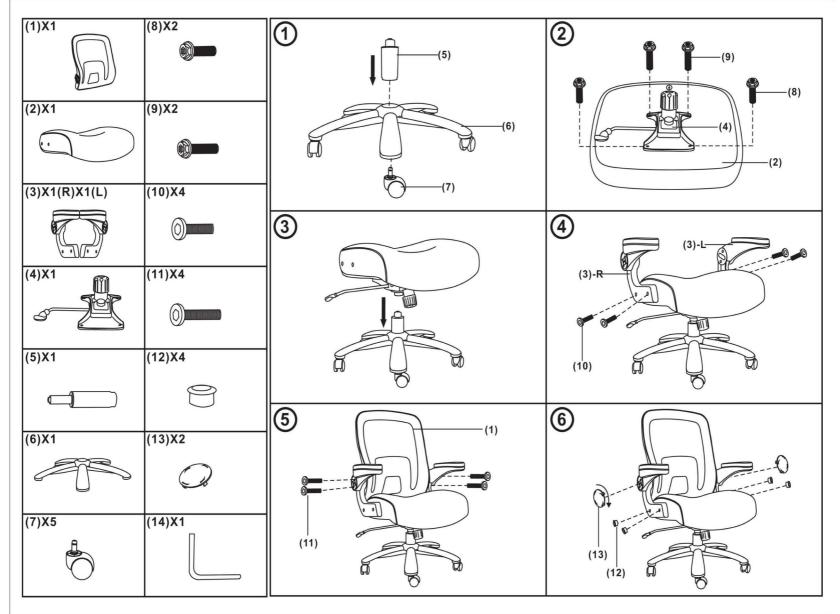
Screws are located in the holes. Use Allen Wrench to back them out for assembly.
